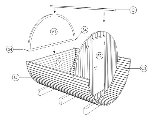
STEP 6: Continue placing body staves (C,C1) tightly on both sides of the sauna using rubber mallet, while fixing body staves on the front panel with screws 4.20x70(S2) and rear window panel (V1) with 4.0 x 50 screws (S3) to prevent glass breakage. To finish the roof top joint, use roof finishing item (H). Different thickness filling peaces (H1) are provided to completely fill the gap.
