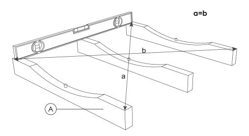
STEP 2: Place the support cradles (A) on level site. The middle support cradle will have no dowel. Carefully level for better stability. Place the center stave (B) on wooden dowels embedded in outer support cradles (A). Fix the center stave (B) with 5.0x100 SS(S1).
