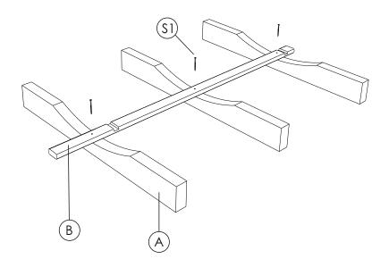
**STEP 3:** Place 6 sauna body staves (C) to each side of the center stave (B) and fix with screws 5.0x100 SS (S1). Be sure to align the panel groove on every next body stave.
