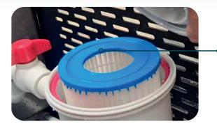
When replacing the filter element, please close the water inlet and outlet valves of the tub, loosen the filter exhaust valve by counter clockwise, then unscrew the filter cover, remove the filter element, and replace the filter element.
