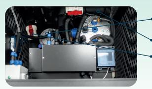
Open the hatch on the top and you can change the filter and open/ close ball valves inside.
